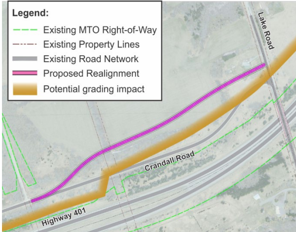
Highway widening may result in grading impacts beyond the existing Crandall Road
