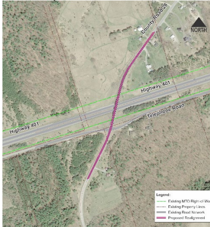
C-6: Replace bridge on existing alignment (road closed during construction with detour via County Road 30 and County Road 41)
